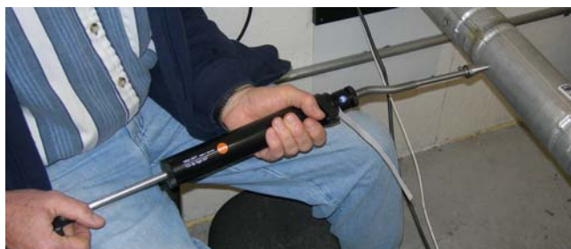
Fig. 4. Testo Smoke Pump for smoke spot test.
