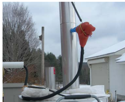
Fig. 3. Heated sampling line for outdoor emissions sampling.
