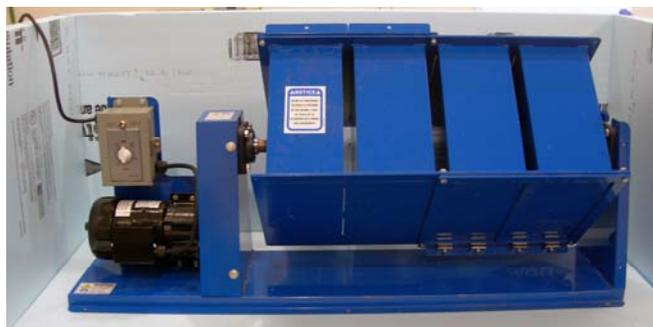
Fig. 3. Pellet Durability Tester.
