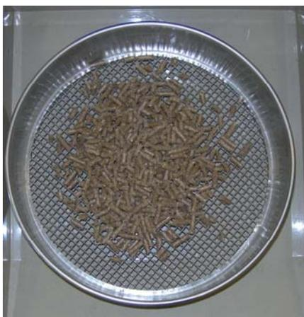
Fig. 1. Screen for determining percent fines.
