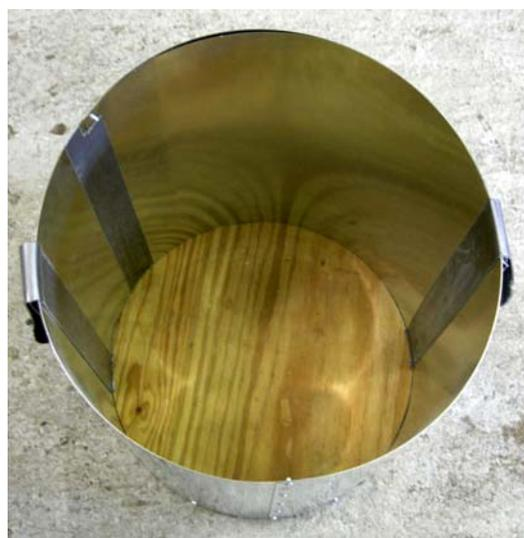
Fig. 2. Container for determining bulk density.
