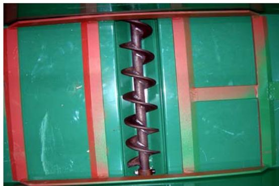
Fig. 3. Bottom of fuel bin, showing auger and moving floor to prevent fuel bridging.
