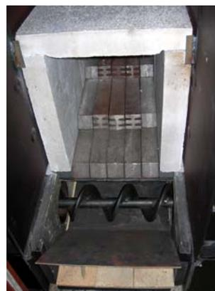
Fig. 2. Moving grate and ash auger.
