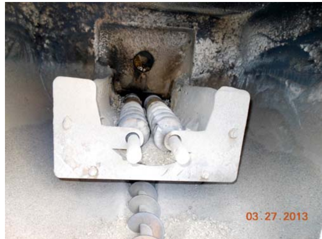
Fig. 2. Pellets drop onto dual augers which slowly move the fuel through the burn pot and down to the bottom, where another auger removes the ash to a storage bin.
