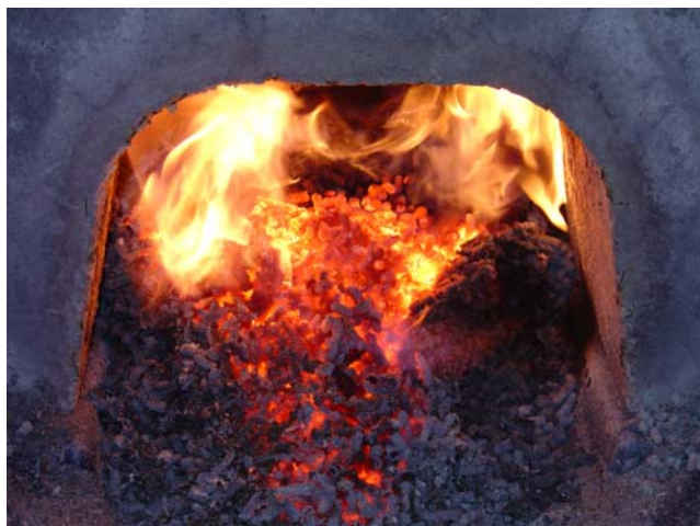
Ash buildup in a pellet boiler.
