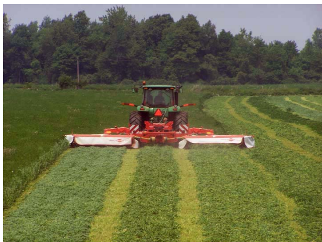
Figure 1. Comparison of conditioned wide vs. narrow swaths vs. unconditioned wide swath using a Kuhn 28' disc mower.
