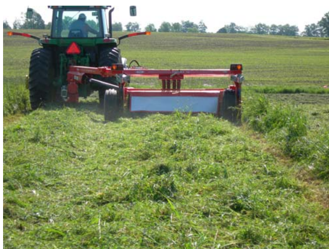
Figure 4. Disc mower with wide swathing attachments producing a swath 100% of the cut width. Alfalfa-grass stand.
